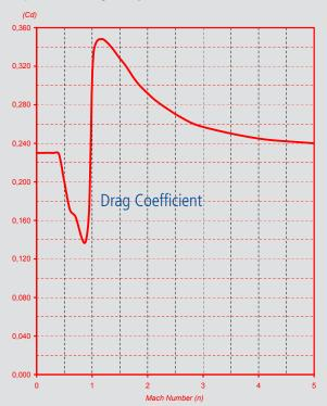
$C_{\scriptscriptstyle D}$  vs MACH data is the basis for accurate trajectory calculation
